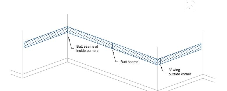
1/8-inch type 304 mill finish stainless steel diamond plate
