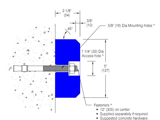
\* Standard bumper is supplied undrilled and with no mounting hardware. Hole spacing shown for bumpers 48" (1219) and longer. Contact factory for hole spacing on lengths shorter than 48" (1219).
